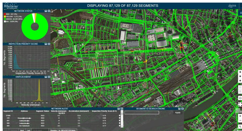
Figure 2 Rheticus® Network Alert User Interface 1 . Example of monitoring of buried pipelines with summary report, trend of instabilities, and filtering tools.
