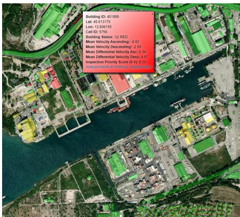
Figure 14 - Detail of the information shown in the pop-up when clicking on a single infrastructure
